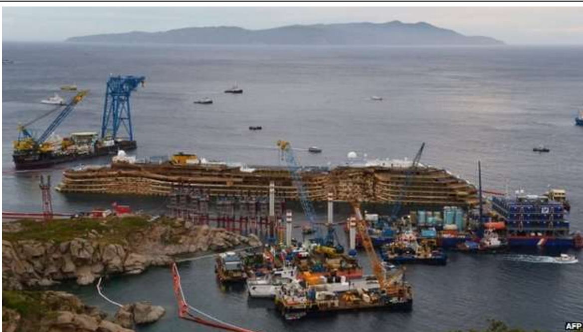
The righted Costa Concordia after the 19 hour parbuckling operation. Photo AFP.
