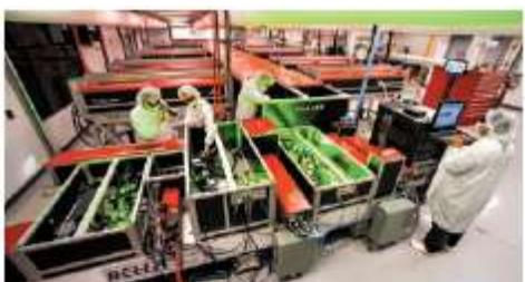
Thales was selected by Berkeley Laboratory in 2009 to develop, realize and deliver the first laser system worldwide with a peak power over 1 PetaWatt (1015 Watt) operating at 1 Hz. The system was entirely developed and integrated within Thales facilities in France, involving a team with skills and competencies in different domains (mechanics, optics, electronics and laser engineering).
