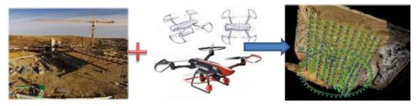
Figure 2. The cloud point generation using unmanned aerial systems
