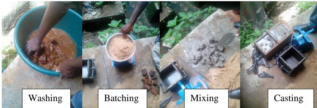
Plate 3: preparation of the specimens (concrete cube)
