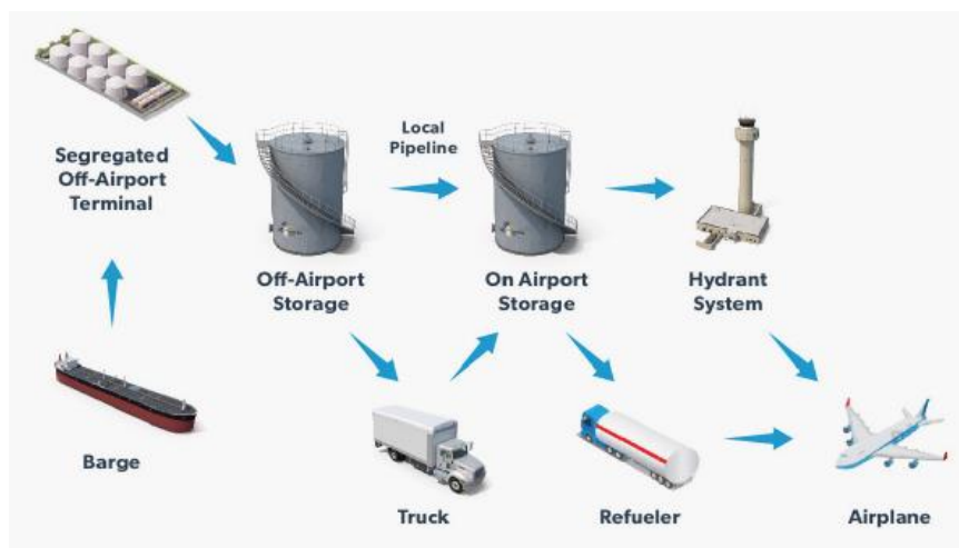
Figure-2 Supply Chain of Aviation Fuel from Segregated off-airport terminal to airplane 4
