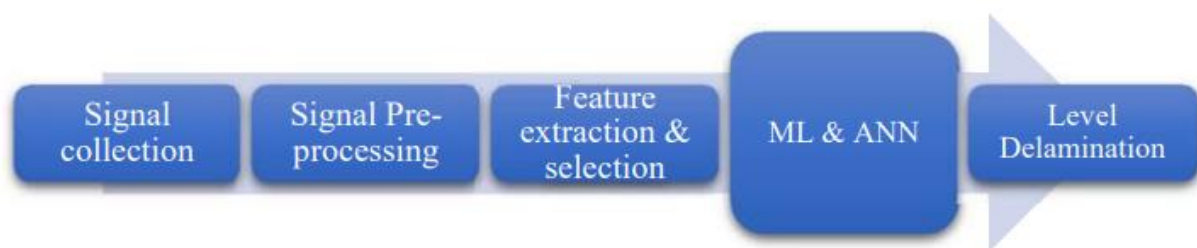
Figure 6 Process for determining the level of delamination in predictive maintenance (Kobbacy, 2012:54)
