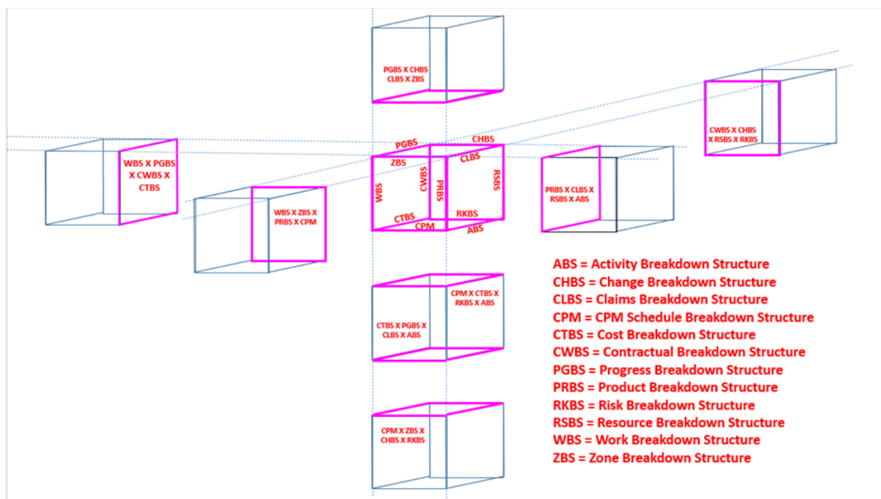
Figure 7. Multidimensional Work Breakdown Structures in Project Management 14
