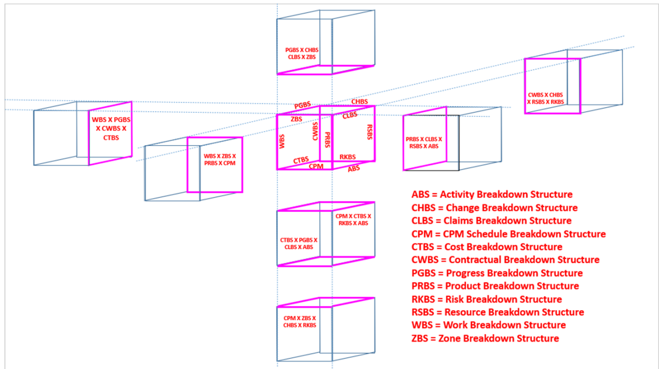
Figure 11 - Multidimensional Work Breakdown Structures in Project Management 30 .
