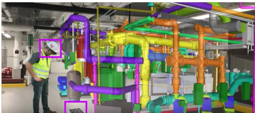
Figure 8 The example of using Augmented Reality in Piping Construction
